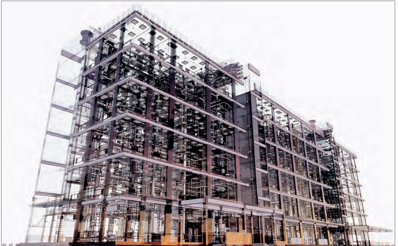
Figure 11: Visualisation of the BIM model of an office building (without the outer skin)
